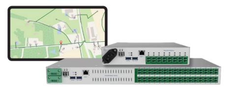
24/7 automated issue detection Monitors up to 64 fibers in 1RU Integrated OTDR and 1xN switch
