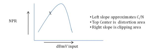
"X "marks the optimum performance spot. The RF dBmV input level at this spot is directly associated with the transmitter OMI value.
