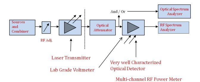
A typical setup for laser transmitter OMI measurement and alignment is shown above. **Note:** Everything to the right of the dotted line is required to set OMI
