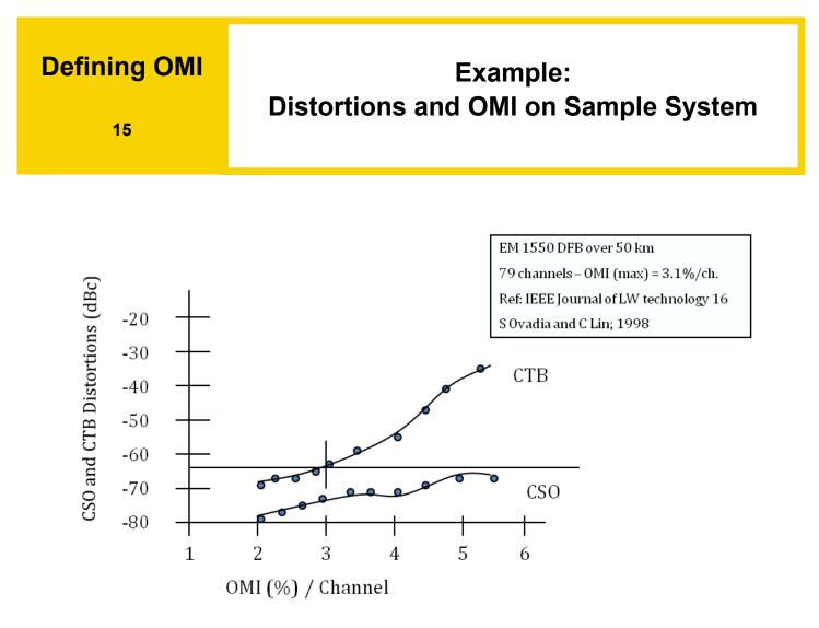
For this example taken from the IEEE Journal of LW Technology, the OMI % per channel provides best performance at 3.1% while maintaining CTB at less than –62 dBc. The total OMI for the 79 channels is 19.5% where m=  $\sqrt{(79 \times m^2/2)}$
