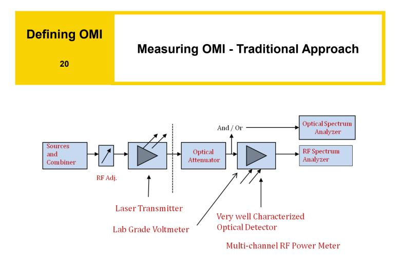
Knowledgeable technicians and very expensive test equipment are typical requirements for determining optimal OMI settings. An RF source with level adjustment capability, a very well characterized optical detector or optical spectrum analyzer, a laboratory grade voltmeter, a multi- carrier RF power meter, and an RF spectrum analyzer to optimize carrier to noise (C/N) are what is required to measure and set OMI.
