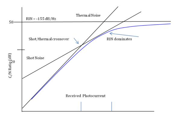
However, in all cases the laser Relative Intensity Noise (RIN) of the laser source limits the overall system performance as the input current to the detector increases (higher light levels). The best operating point for the receiver is at or slightly beyond where the RIN begins to dominate. At this point the system performance hits a point of diminishing returns as shown by the composite curve. For detector current this is typically at around 0 dBm or 1 milliamp detector photo current.
