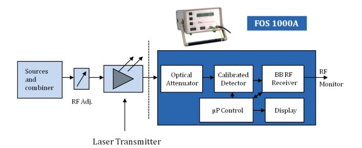
A typical setup for laser transmitter OMI measurement with the FOS 1000A instrument. *Note:* FOS 1000A replaces all required equipment using the traditional method
