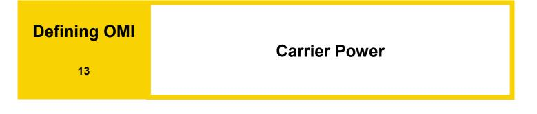
Carrier power in multi-channel optical systems is defined as one half the square of the optical modulation index (m) times the optical power (P or IR).
