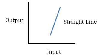
For example, if the input is current to a laser and the output is light, the light intensity output will be very linear (as shown by the straight line) and the light would represent the drive signal very well. In this case, the straight line would be a part of the transfer curve of the laser.
